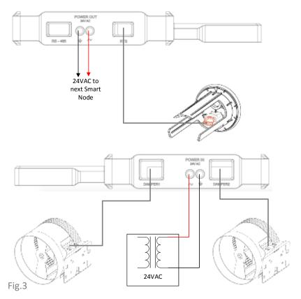
Remote Temperature and Humidity Sensor (RTH) Harness. Both ends of the RTS harness are the same male connectors. Run one of
