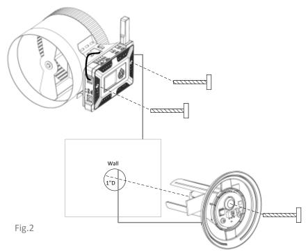
Mounting the Smart Node. To Mount the 75F Smart Node, first identify the primary damper in the zone. If there is only one damper, that is the primary damper. If there are two, pick the most accessible damper as you will need access to the Smart Node. Using the provided hex key bolts, screw the Smart Node to the damper side bracket cage nuts until snug.
